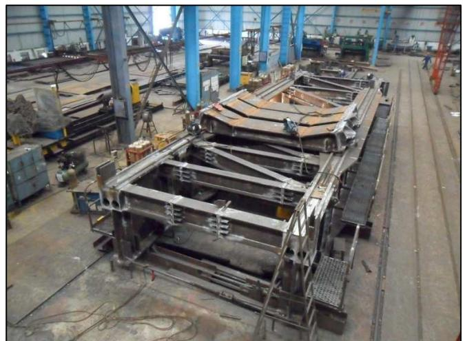
**Figure 4 – Trial assembly of Steelwork in the factory**
