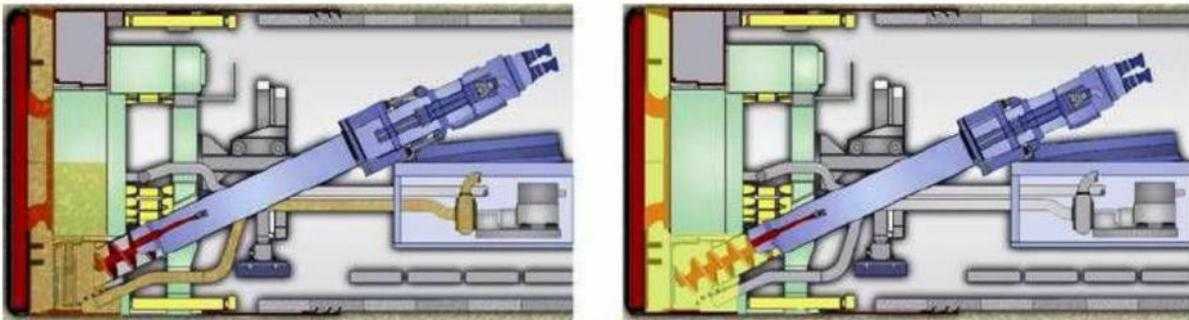
Figure 8. The Socatop TBM in Slurry Mode (left) and EPB Mode (right)
