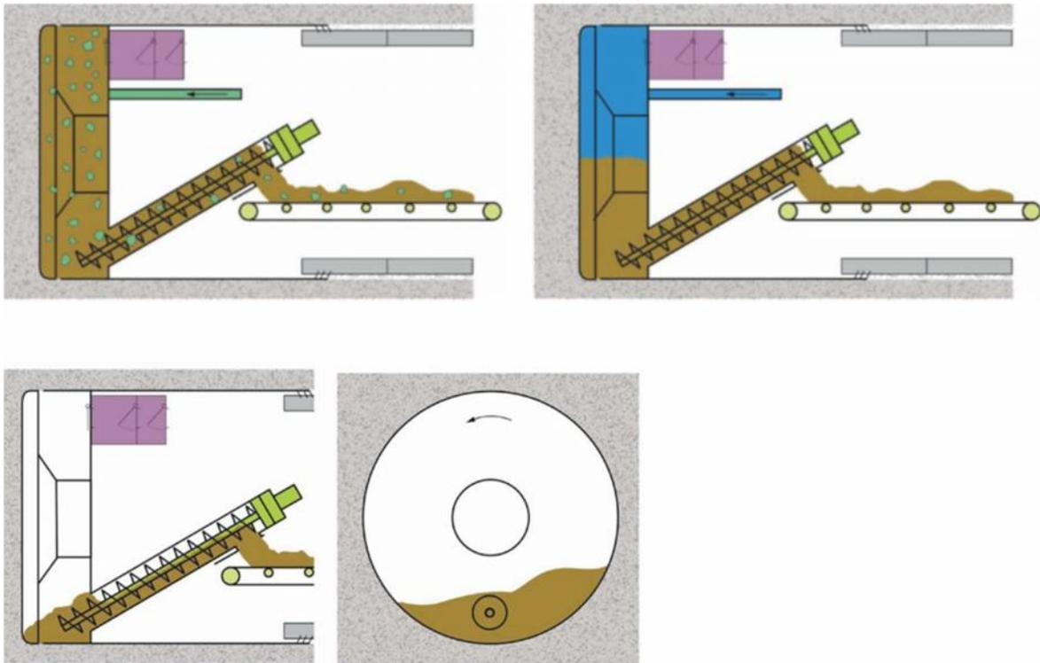
Figure 4. Different Operation Modes of EPB machines
