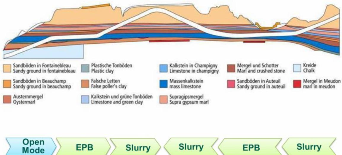
Figure 2. Changing geology conditions of the Socatop Project
