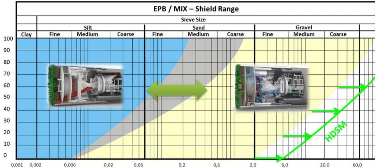
Figure 9. The extended application range of the variable density TBM
