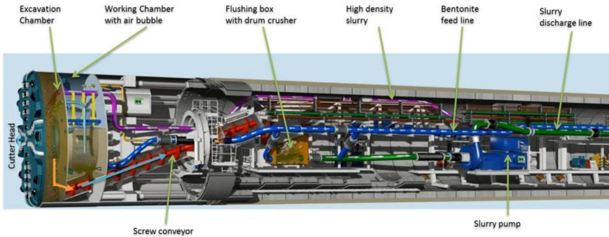
Figure 10. The Variable Density TBM (shown with hydraulic transport)
