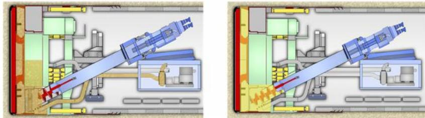
Figure 3. Modular and integrated convertible machine principles
