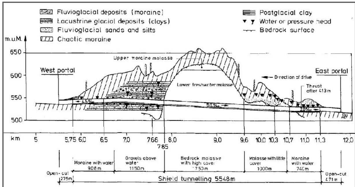
Figure 7. Longitudinal cross section of the Grauholztunnel
