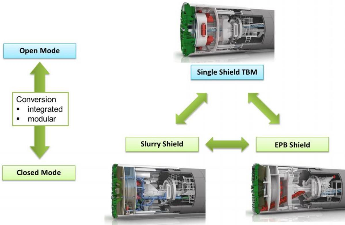
Figure 1. Different possibilities for conversions of TBM types.
