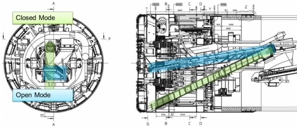
Figure 5. Integrated Convertible EPB / Open Shield TBM for the Saverne Tunnel
