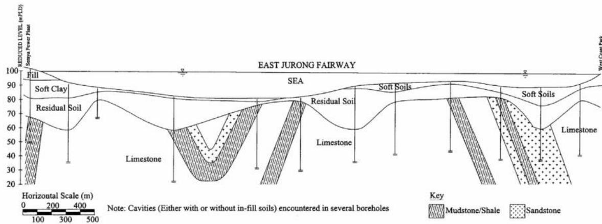
Figure 12. Possible Geology Alignment with Limestone in Jurong Formation
