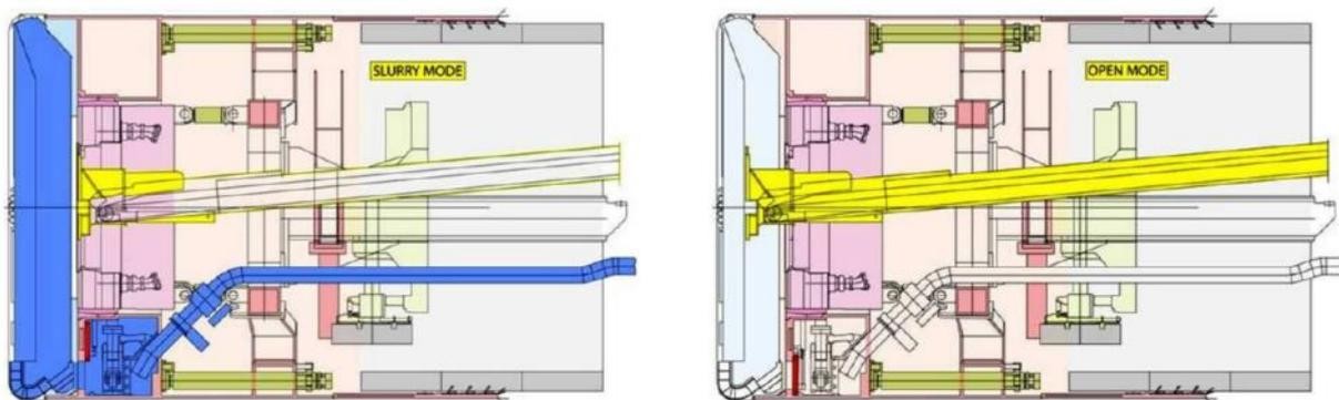
Figure 6. Convertible TBM in Mixshield Mode (left) and Open Mode (right)
