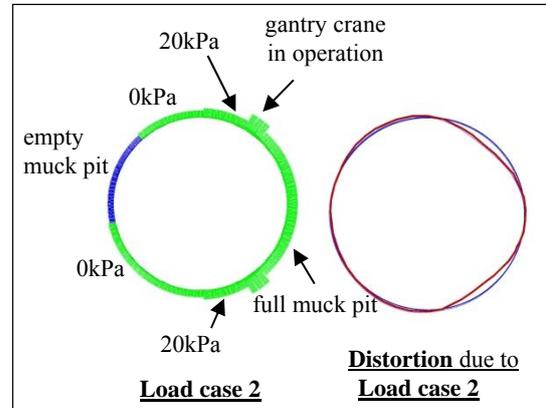
Figure 3. Additional distortion due to Load case 2 in Table 3
