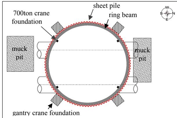
Figure 2. Typical site utilization plan
