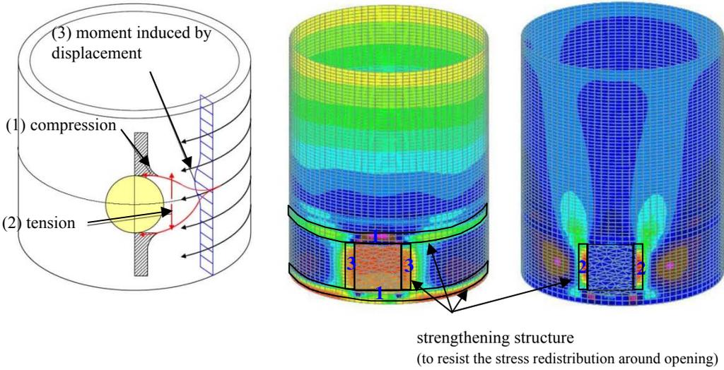
Figure 4. Stresses around opening and its strengthening system
