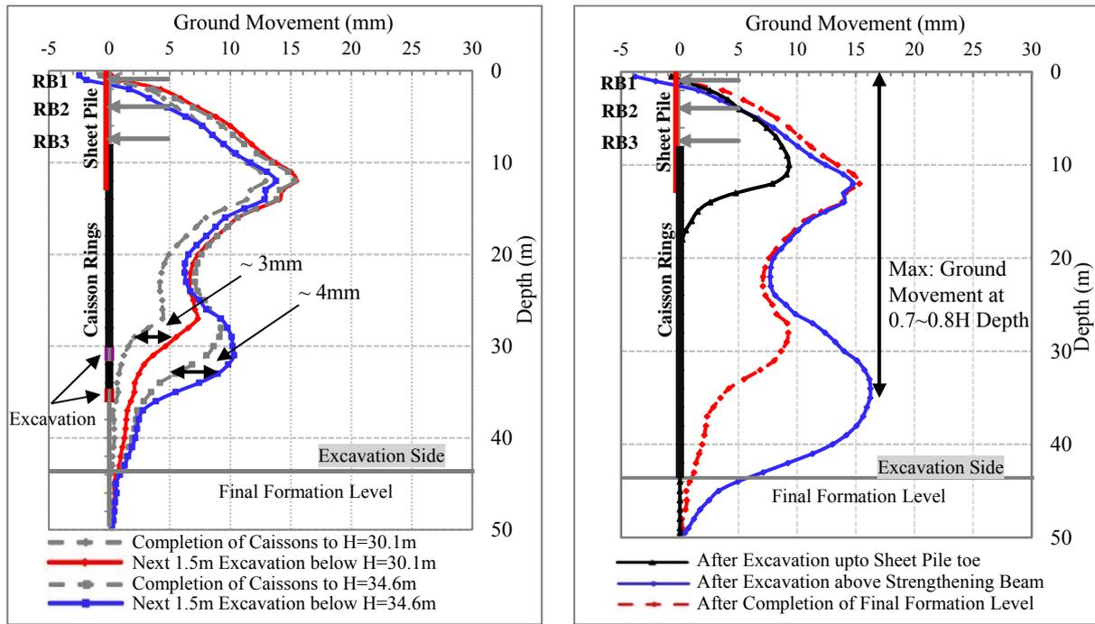
(a) Ground movement behind completed ring above due to next 1.5m excavation below
