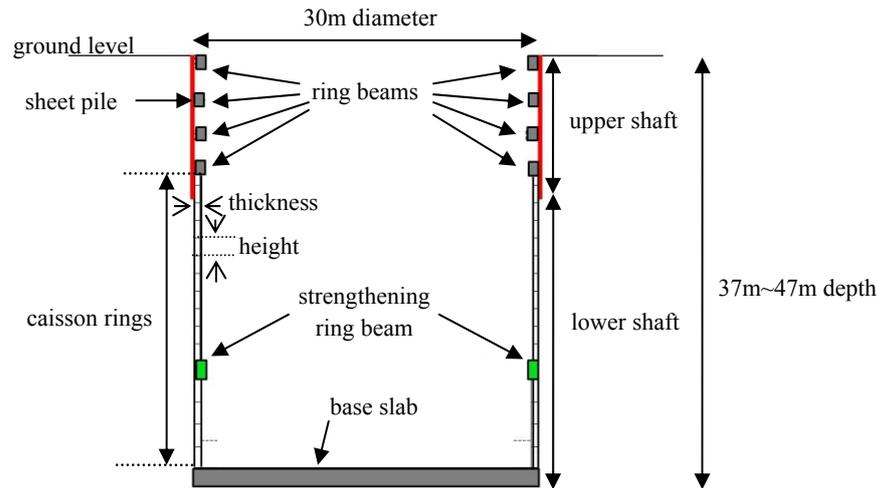
Figure 1. Typical support system of circular shaft
