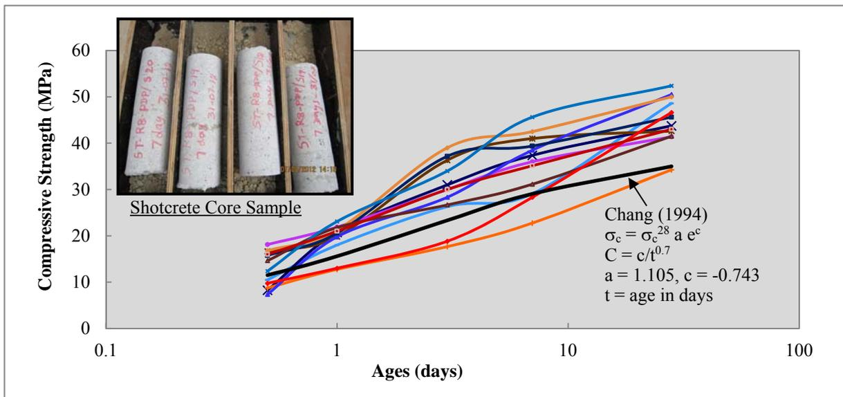
Figure 11. Recorded shotcrete compression strength with time
