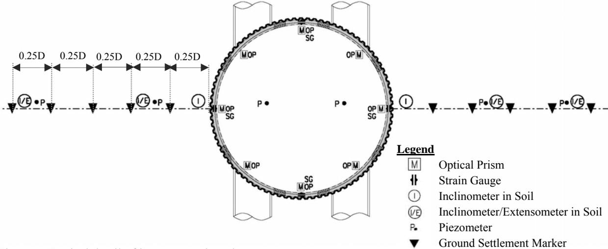
Figure 5. Typical detail of instrumentation plan
