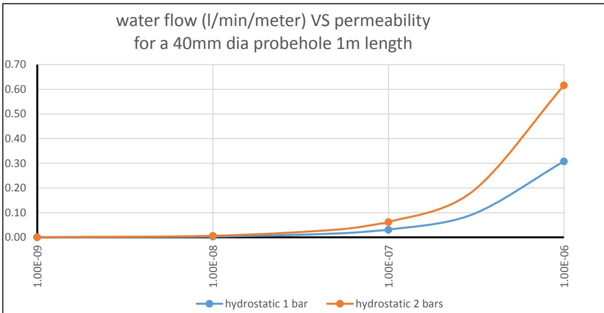
Figure 27: Graph of Water Ingress against Permeability for 1bar and 2 bar hydrostatic pressure
