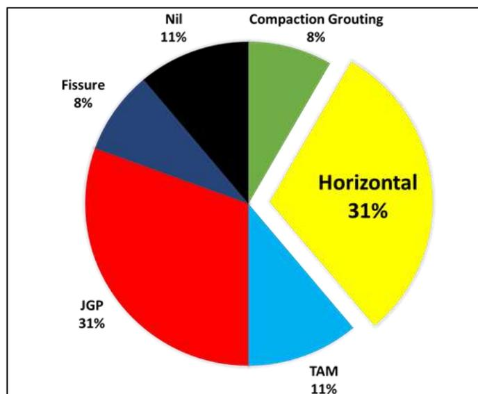
Figure 6: TELC1-C2 summary of grouting method for the 34 CPs
