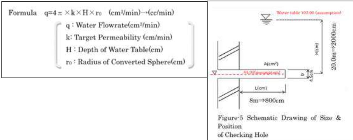
Figure 26: Formula for the determination of the allowable flow rate for a given permeability “k”
