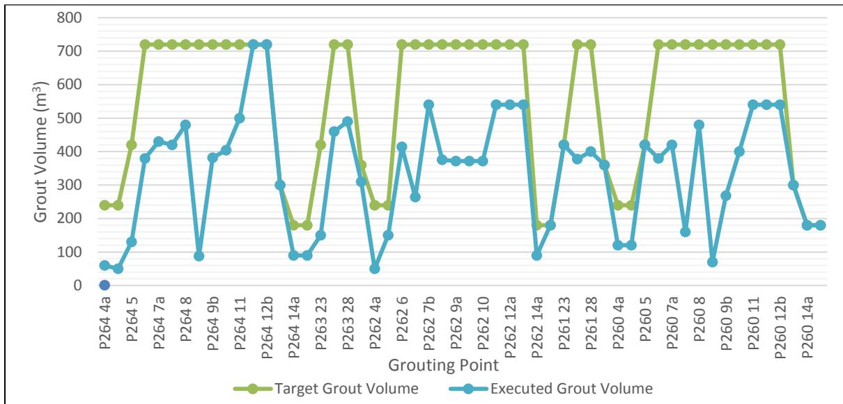
Figure 20: Grout Point vs Grout Volume Graph for Target Grout Volume and Executed Grout Volume for Adit Tunnel
