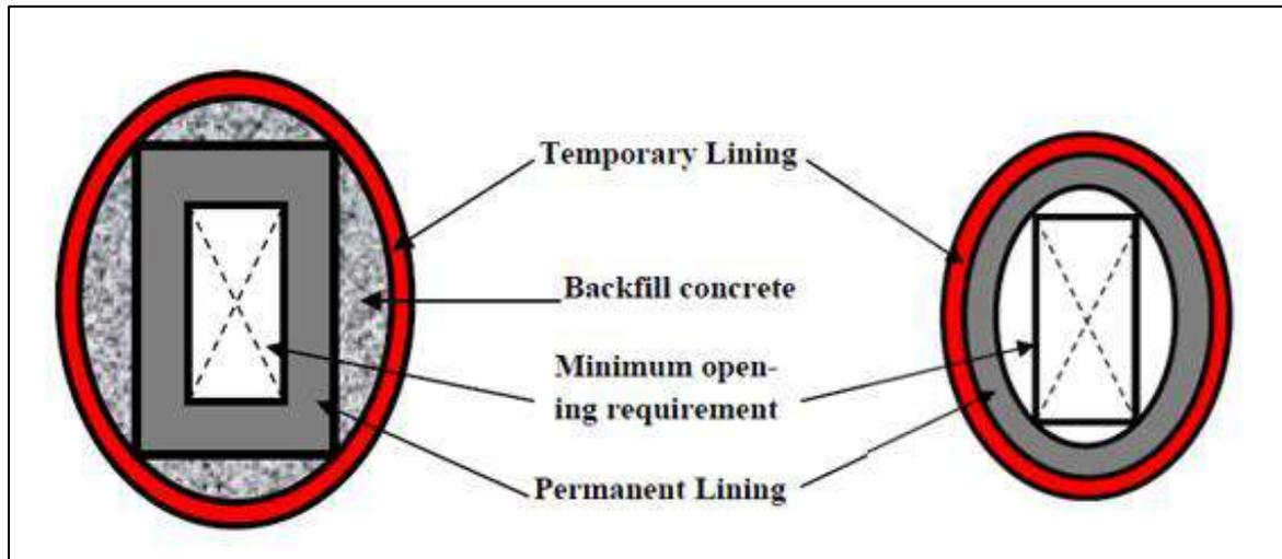
Figure 9: Rectangular and Oval permanent lining
