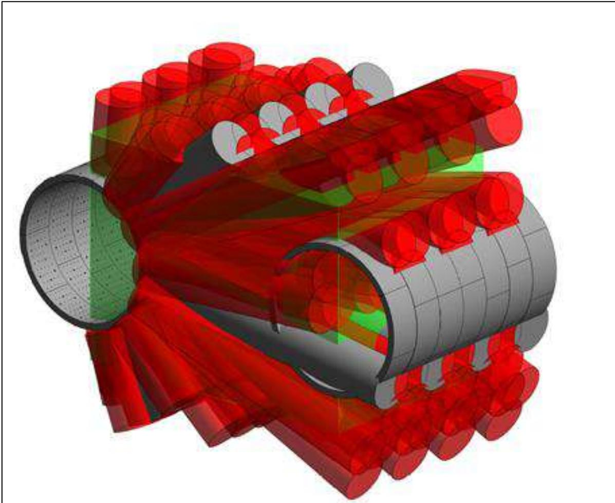
*Figure 15: Coverage of horizontal grouting using the additional grout ports*
