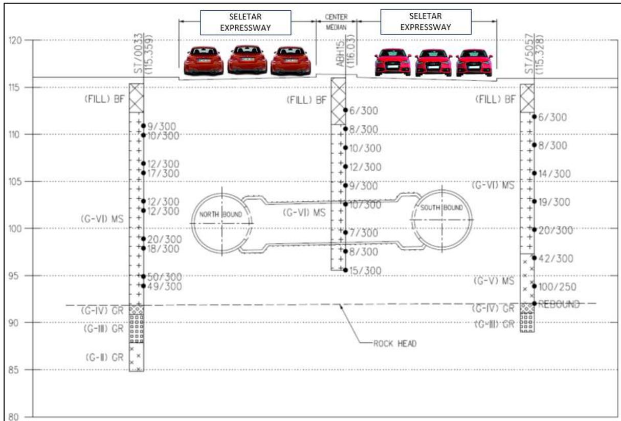
Figure 16: Cross section of Cross Passage 3 (CP3) under Seletar Expressway
