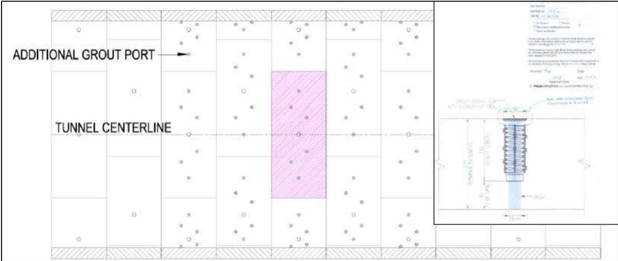
Figure 12: T211 Grout port arrangement, profile of bored tunnel
