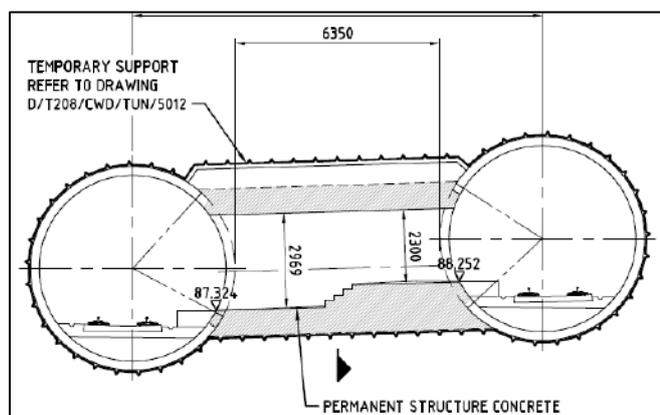
Figure 10: T208 CP profile, constant "collar" section
