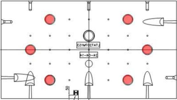
With the usage of the additional grout ports, there is a great extent in the potential geometrical coverage of the horizontal grouting done from the bored tunnel.
