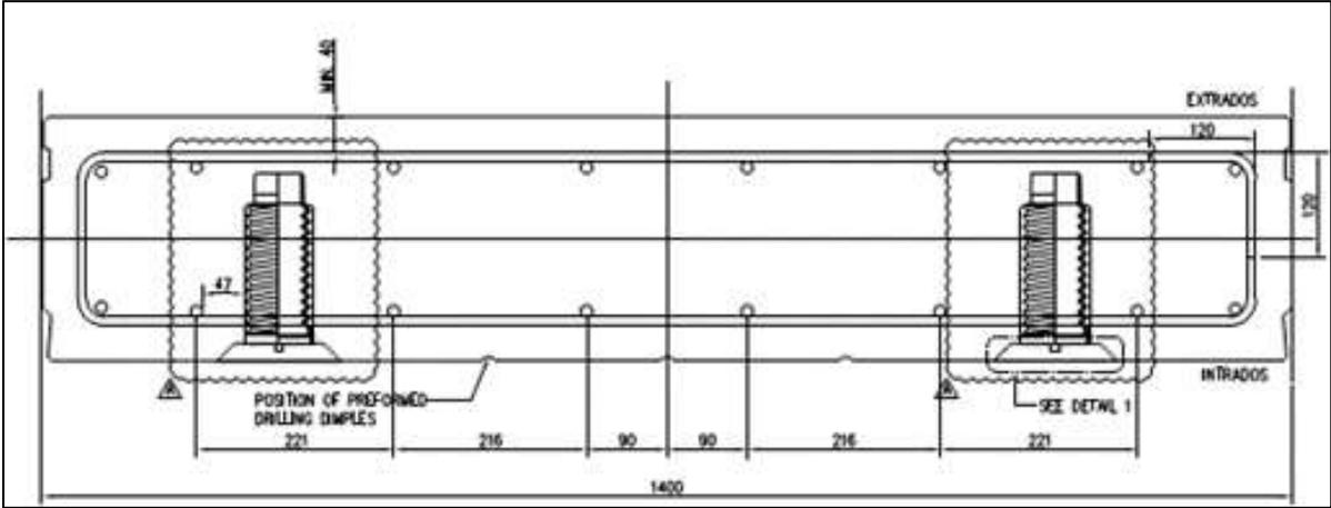
Figure 13: T207 Additional grout socket arrangement
