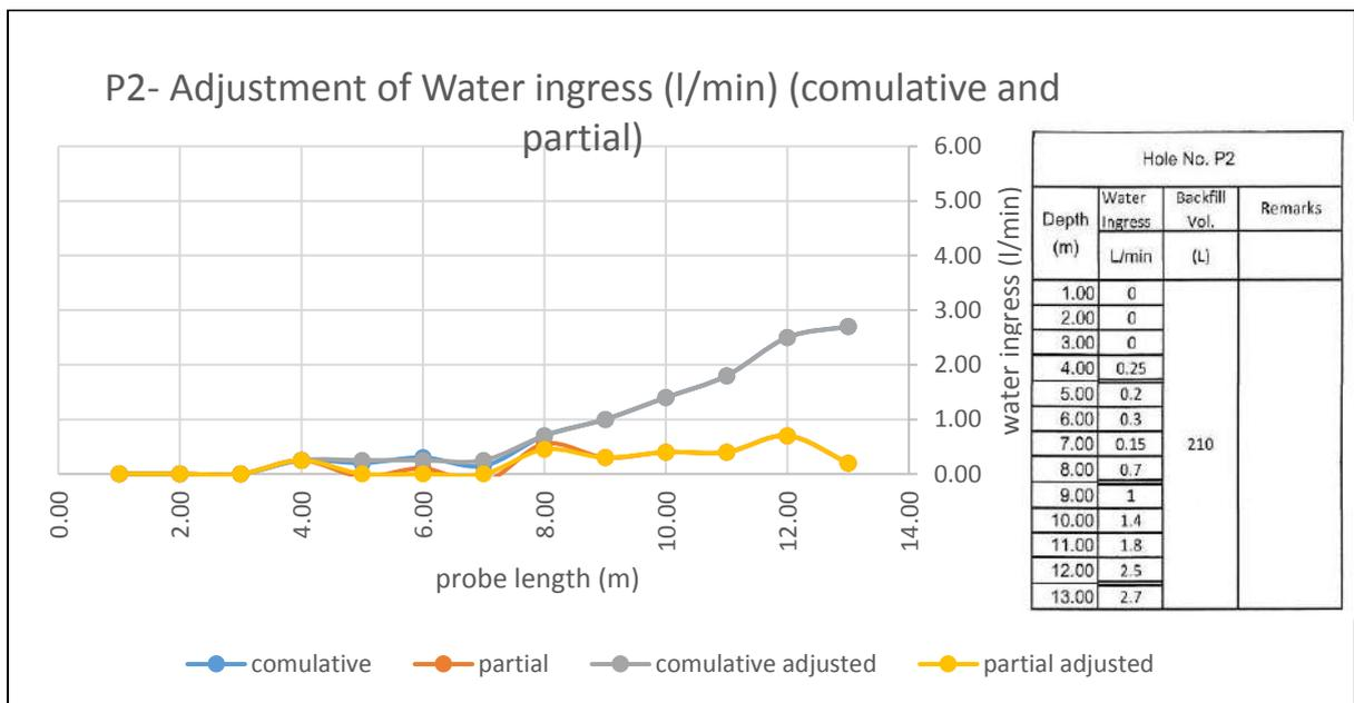
Figure 23: Water ingress with respect to depth
