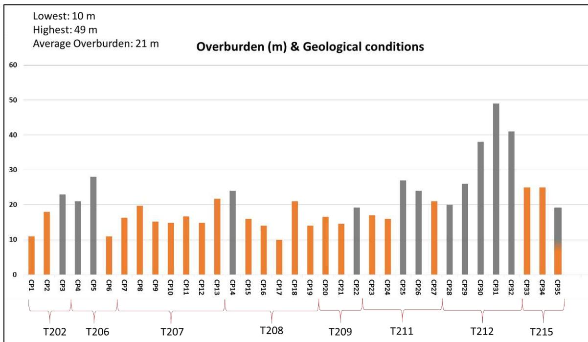
Figure 4: TELC1-C2 summary of CP overburden and geological conditions
