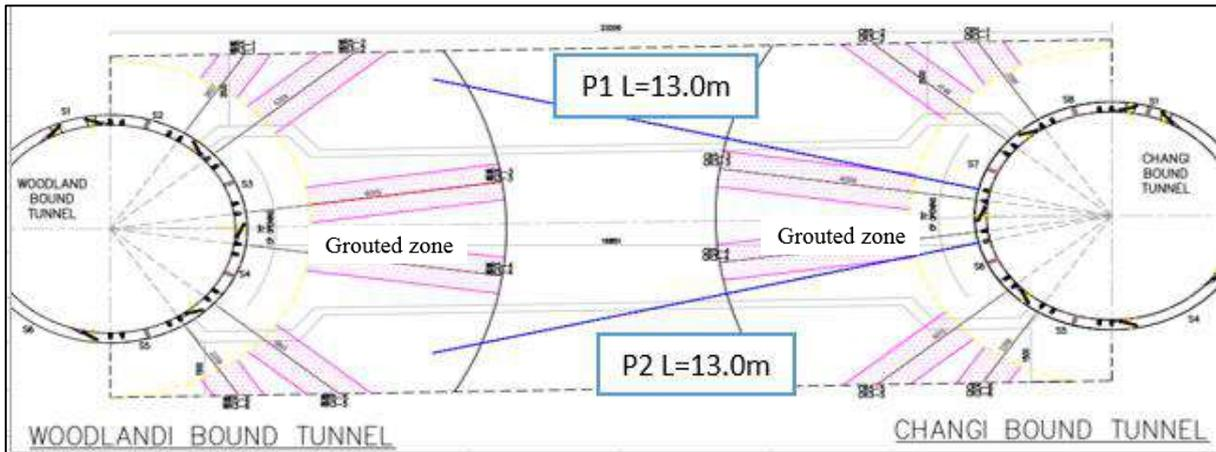
Figure 22: Probe Drilling from Changi Bound for CP3
