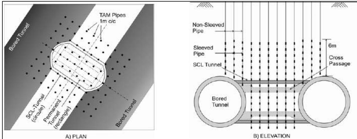
Figure 7: Typical vertical grouting scheme for Cross Passages
