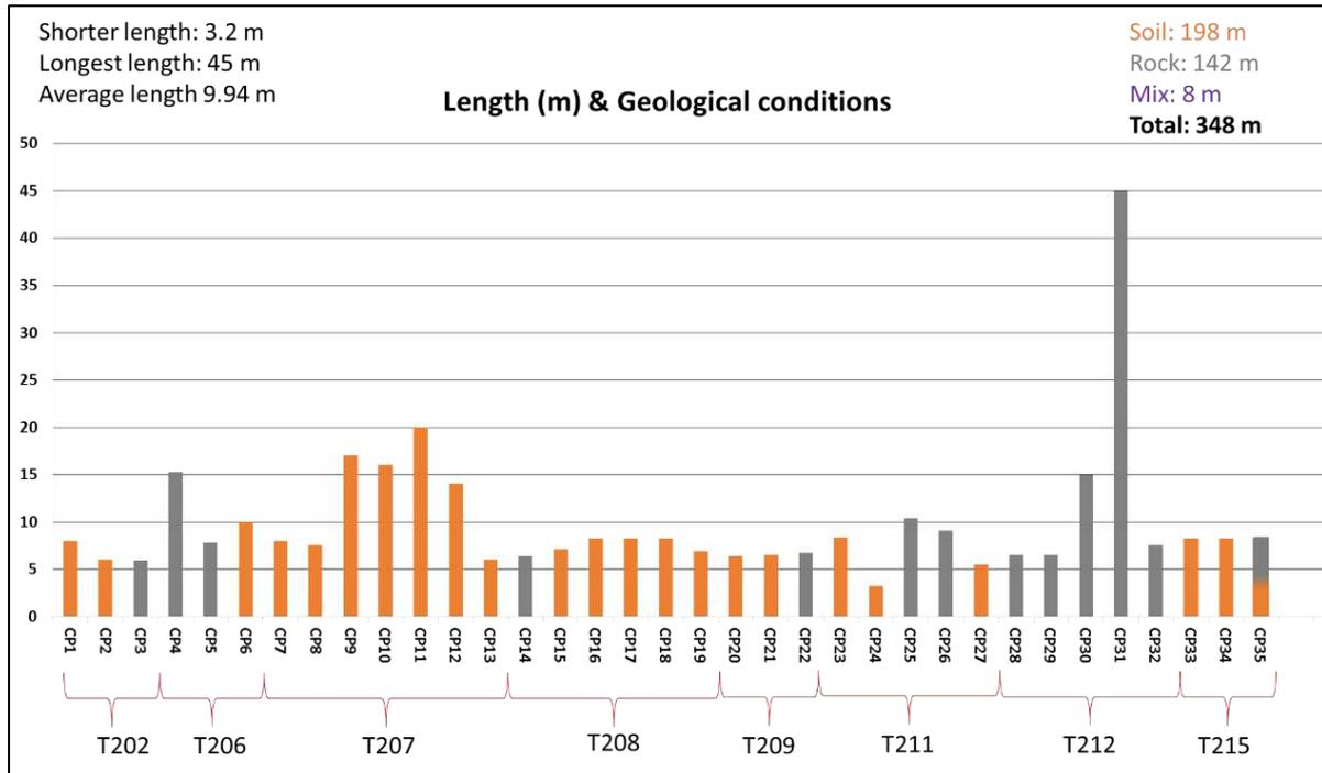
Figure 3: TELC1-C2 summary of CP length and geological conditions
