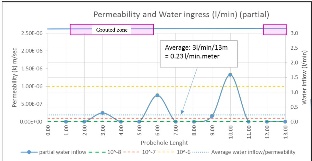
Figure 24: Probeghole P2 - Permeability and Water Ingress chart
