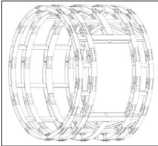
Figure 111: Typical bracing for bored tunnel.
