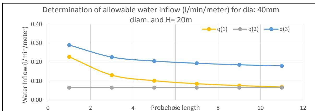
Figure 28: Comparison of formula for the determination of allowable water inflow
