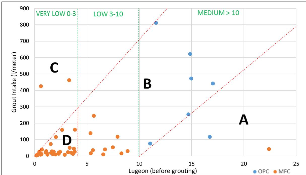
Figure 25: Graph of Grout Intake (Ordinary Portland Cement and Microfine Cement) VS pre-grout Lugeon value
