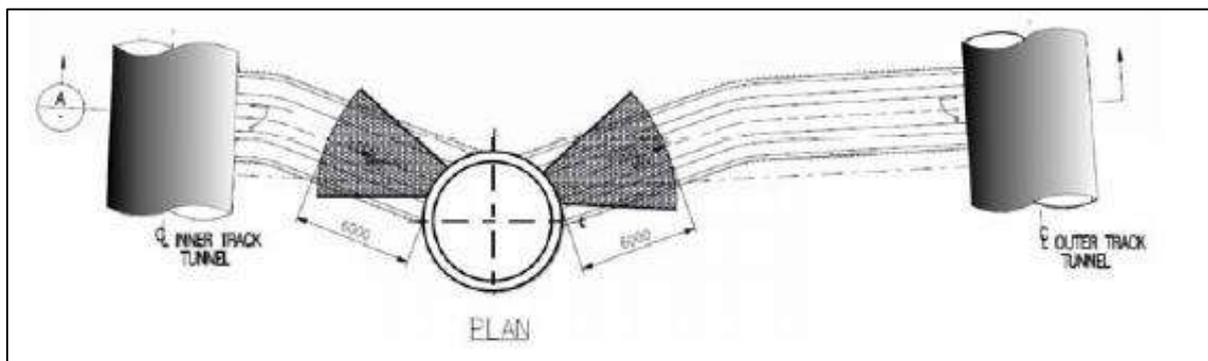
Figure 8: C855 CP1 horizontal grouting (stage 1)
